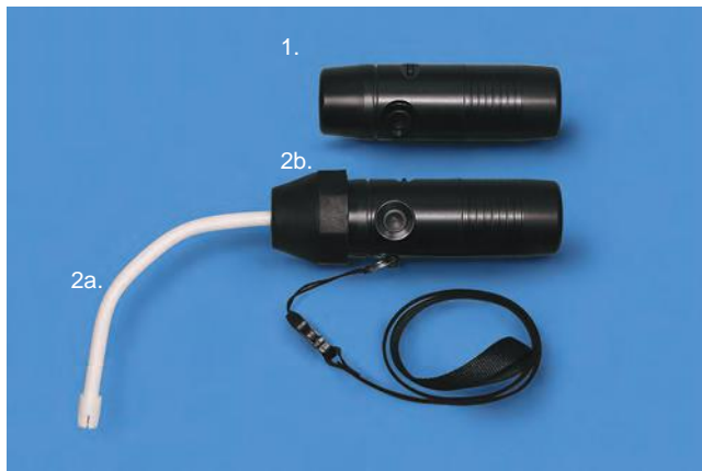
Figure 39.5 An artificial larynx. This device is a sound generator. Item 1 is shown without an attachment/attenuator and can be used with neck placement or cheek placement. When used this way, sound is directed through the neck or cheek tissue into the oral cavity. Item 2 is shown with an intraoral attenuator (2a) and an attachment (2b). Together, the attachment and attenuator allow for the delivery of sound into the oral cavity, which can then be shaped into speech.
